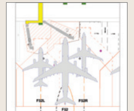
MARS layout at aircraft stand F52
